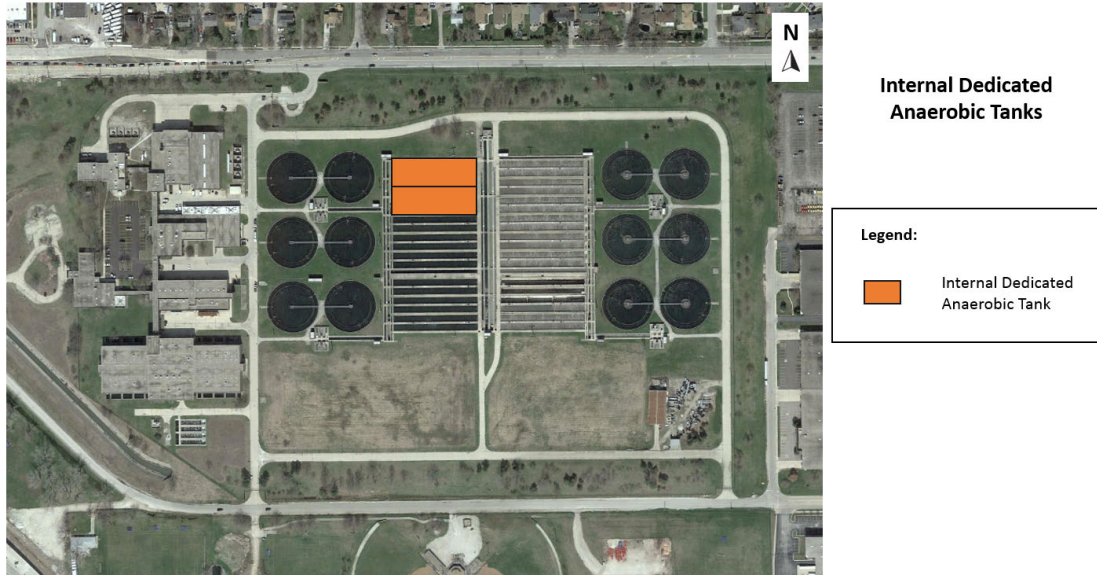
Figure A.2.10 Alternative 1.II - Retrofit of Existing Battery B Aeration Tanks into Dedicated Anaerobic Tanks
