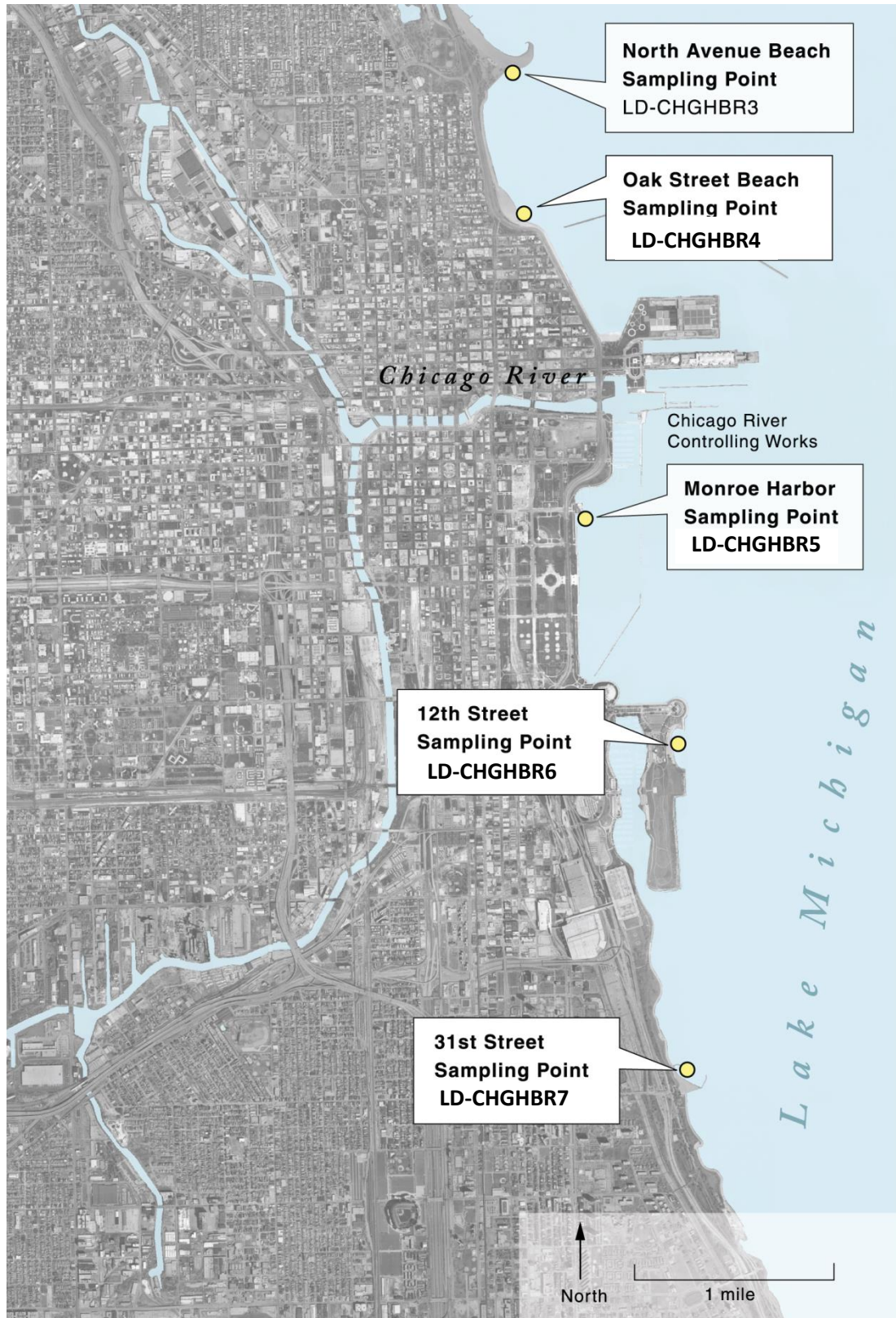
FIGURE 4D.2: LAKE MICHIGAN BEACH SAMPLING LOCATIONS FOLLOWING CHICAGO RIVER BACKFLOW
