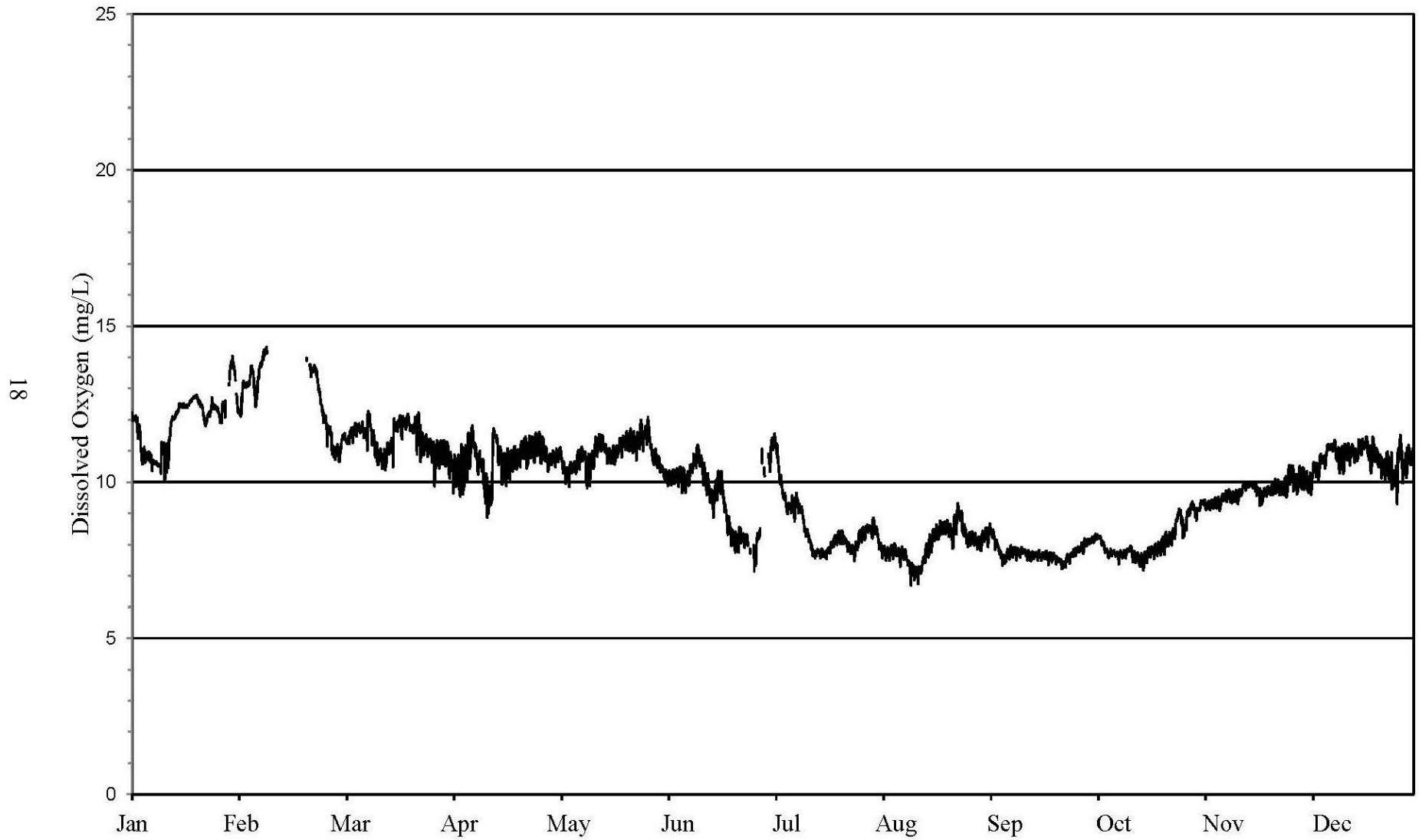
FIGURE 6: DISSOLVED OXYGEN CONCENTRATION MEASURED HOURLY AT MICHIGAN AVENUE ON THE CHICAGO RIVER FROM JANUARY 1, 2021 THROUGH DECEMBER 31, 2021
