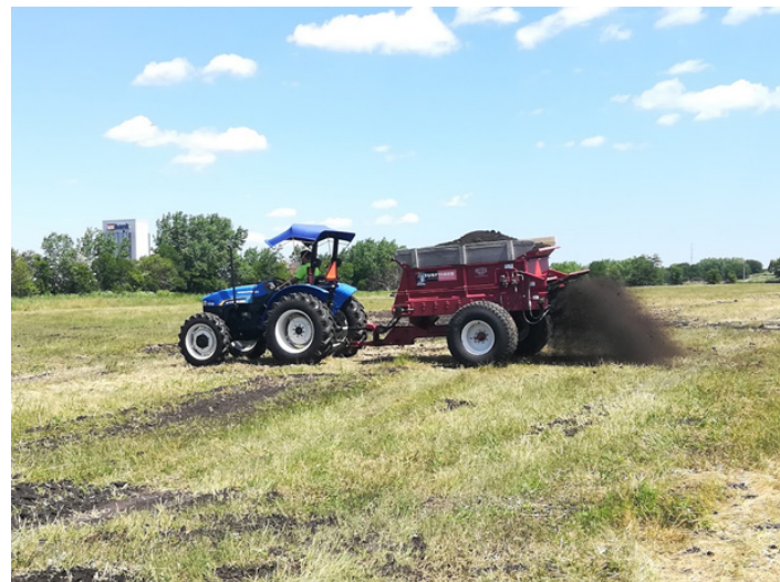
Photo of Tiger spreader topdressing a field with biosolids at a 1/2" rate.
