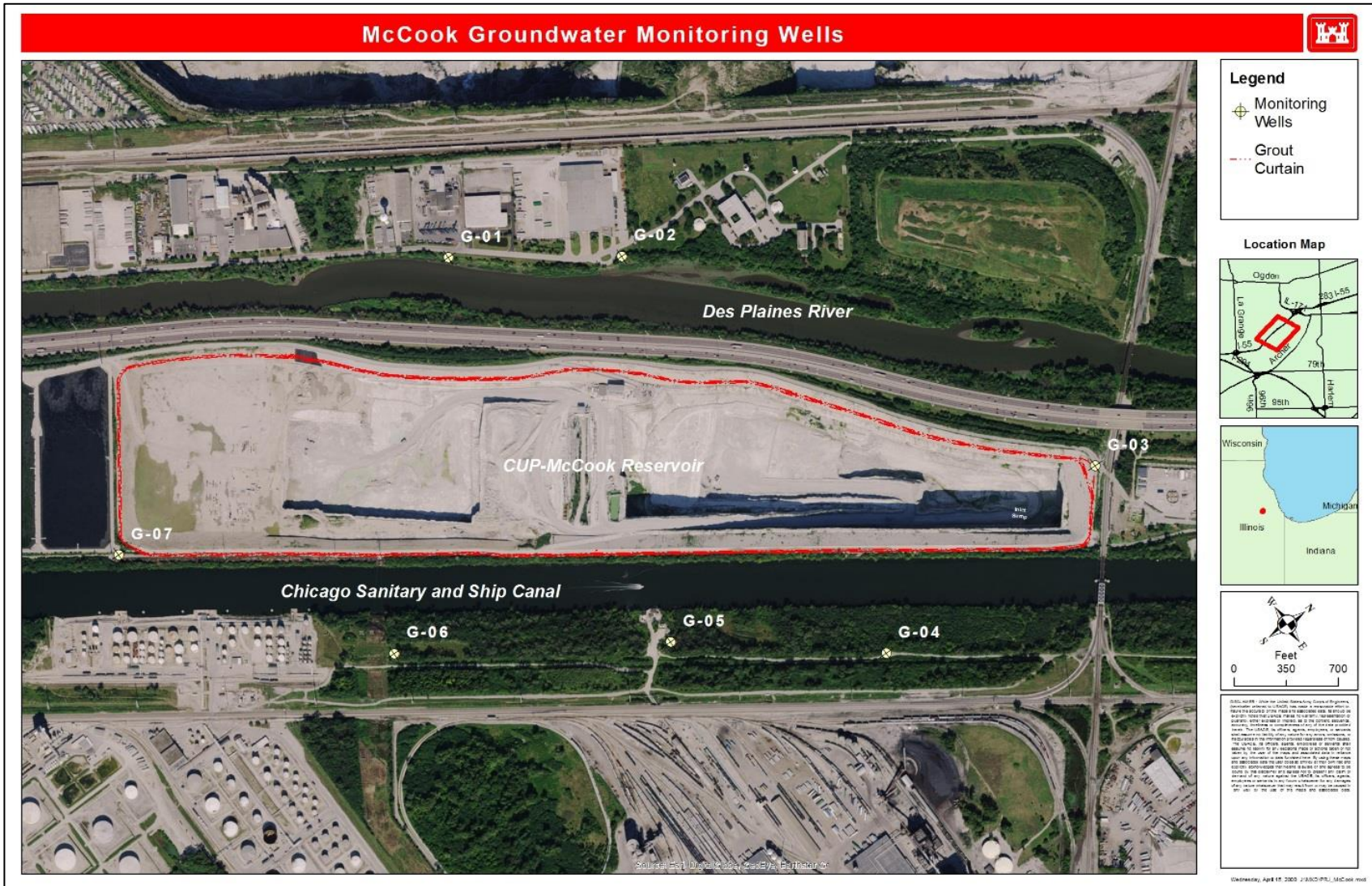
FIGURE 1: McCook Reservoir Site and Monitoring Well Locations
